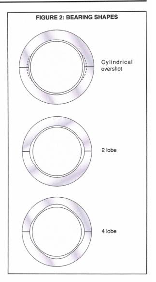
lindrical-overshot bearings (the sleeve bearings most common to electrical machinery) the upper peripheral speed limit is approximately 6,000 ft (1,830 m) per minute. Higher speeds require special designs, starting with 2-lobe, then 4-lobe bearings, as well as special lubrication methods (Figure 2).
